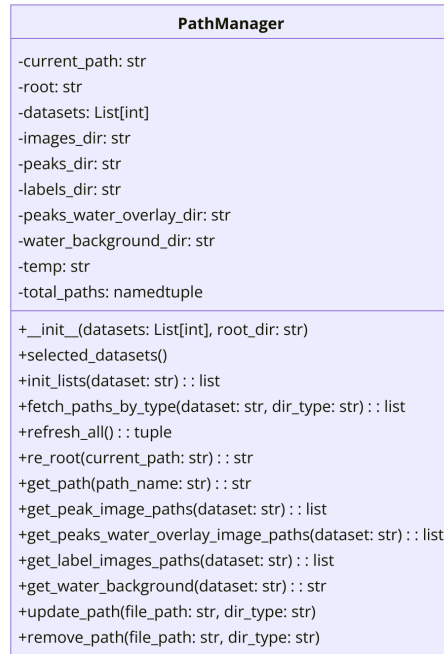
Figure 9: path.py UML diagram
