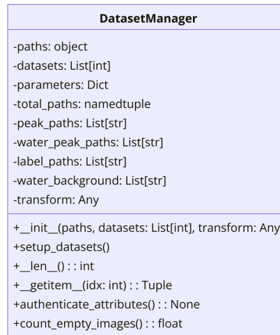
Figure 10: data.py UML diagram
